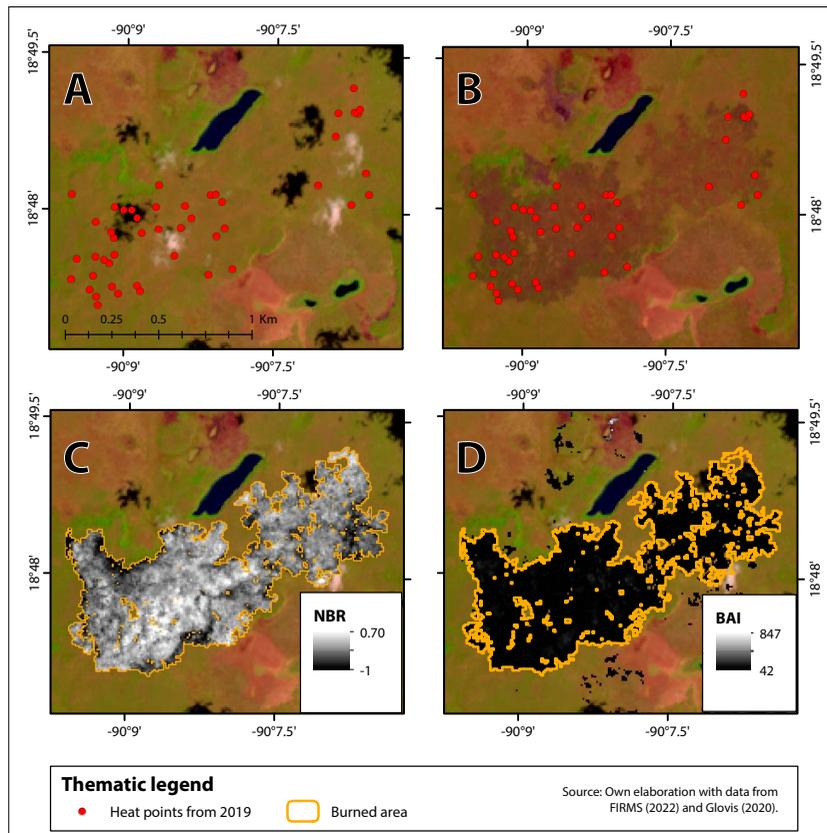
Figure 2. Processing of burned areas. Images A (pre-fire, March 24, 2019) and B (post-fire, April 25, 2019) show the false-color RGB 754 compounds in Landsat 8. Red shows the heat spots (VIIRS). Images C and D show the NBR and BAI indices generated with the post-fire image of April 25, 2019. The orange line marks the final perimeter of the burned area.
