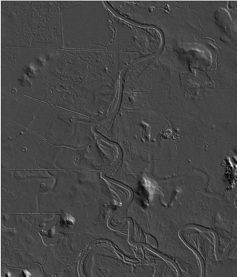
Figure 6. Improved LiDAR DTM resulting from local transformations.
