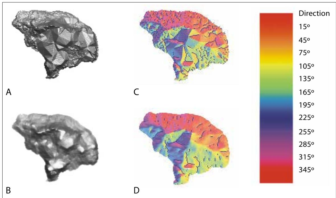
Figure 7. DTM Hillshade: A, original DTM, B, corrected DTM. Aspect and drainage network extraction. C, original DTM and D, corrected DTM.
