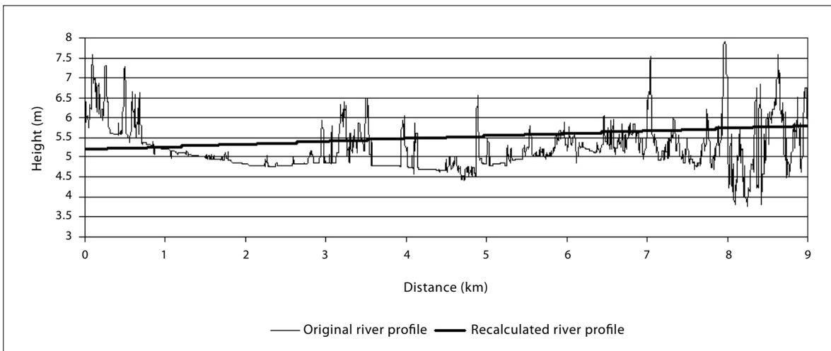
Figure 9. River surface profile following the skeleton.
